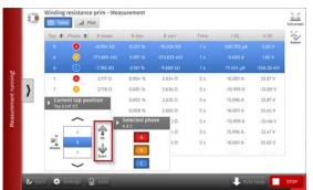
Set Automatic tap control to **OFF** in Settings view: Switch taps manually using TouchControl while a measurement is running.
