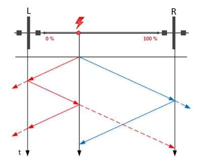
Figure 3: Bewley lattice diagram showing the propagation of traveling waves over time
