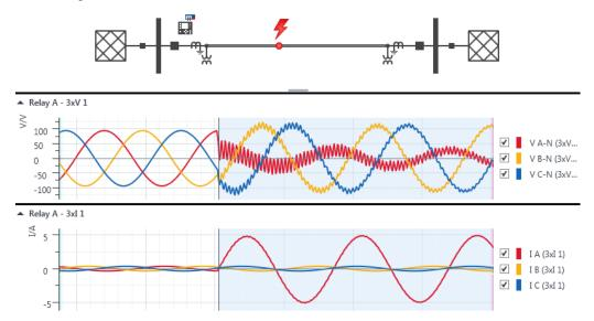
Figure 7: Network simulation of a single phase to ground fault on a 100 km transmission line using a lumped RLC model
