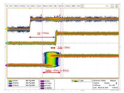
Figure 9: Jitter of traveling wave pulses for two time-synchronized distributed test devices
