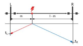
Figure 5: Two-ended fault location based on time difference of first arrival times
