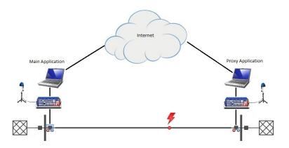
Figure 8: Setup for an end-to-end test using distributed test set synchronized using GPS
