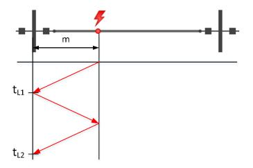
Figure 6: Single-ended fault location based on time difference of first arrival and first reflected waves
