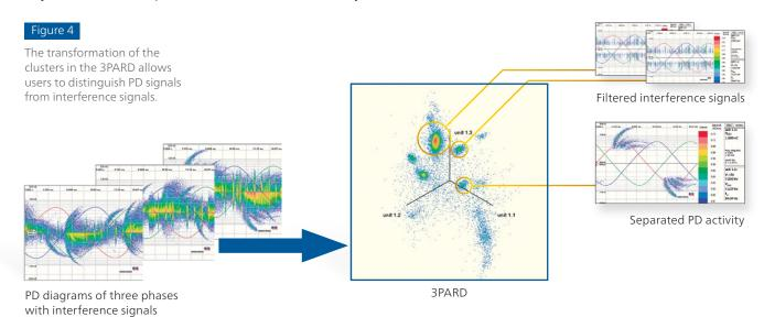
The combined results of three measurement channels are displayed in a single 3PARD star diagram, which facilitates result comparison and separation of impulse sources. To further increase the testing reliability, clusters are selected in the 3PARD and the resulting PRPD diagrams show the filtered-out pulses in real time while graying out the residual pulses in the background (Figure 5).
