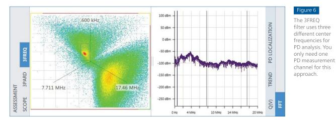
Using a 3FREQ diagram, you can separate PD events such as surface discharge, corona and internal voids from disturbances. Just as with the 3PARD, the resulting PRPD diagram shows filtered out pulses while graying out the residual pulses in the background to improve the testing reliability.
