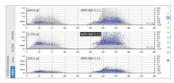
Filtered PRPD diagrams based on a 3PARD back transformation and the gray residual pulses.
