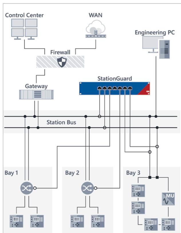
Figure 2: Structure of a substation with connected IDS
