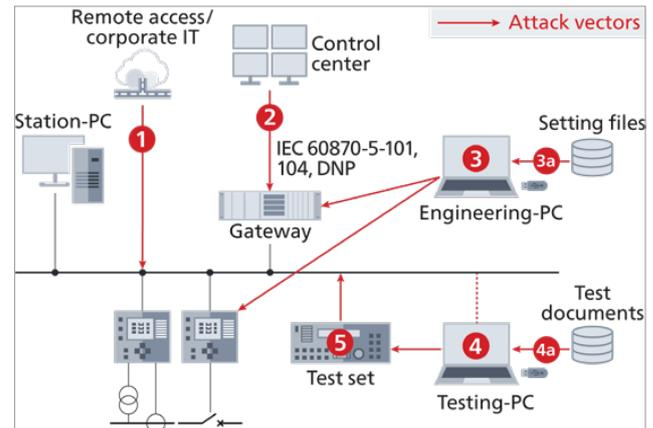
Figure 1: Attack vectors of a substation
