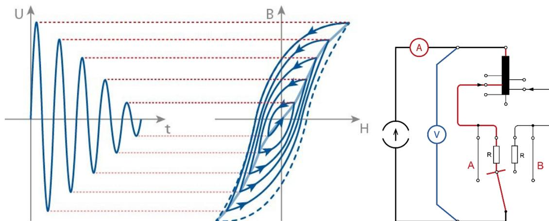
Figure 1: Demagnetizing the transformer core with sinusoidal signal
