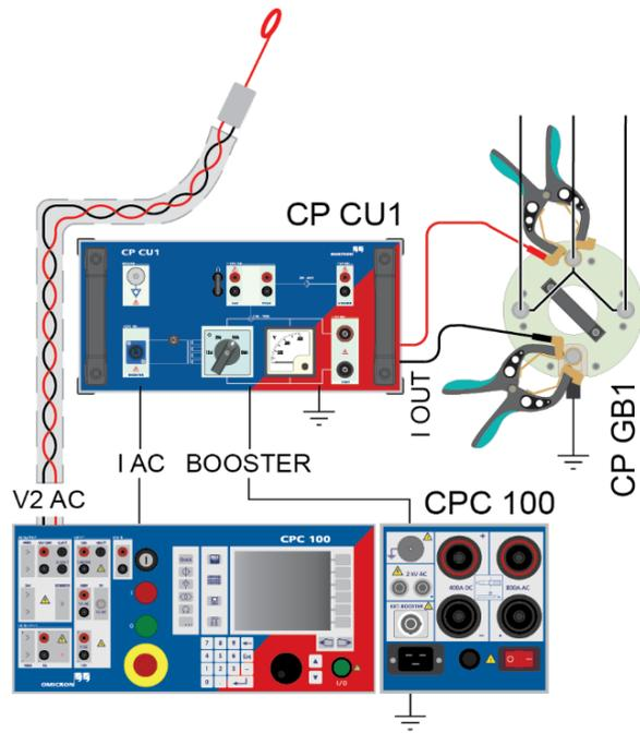
Figure 9 - Test setup with CPC 100, CP CU1, CP GB1 and a current clamp
