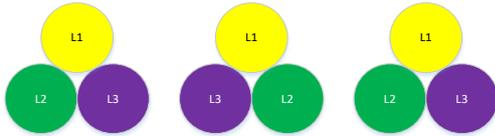
Figure 4 - Parallel single-core medium-voltage cables after crossing out
