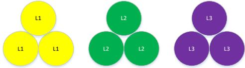
Figure 3 - Parallel single-core medium-voltage cables when connected to a switchgear or other equipment
