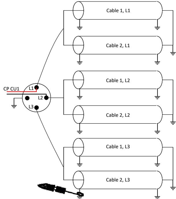
Figure 12 - Supply at L1-L2 and measurement at shield of cable 2, L3
