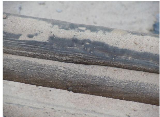
Figure 7 - The sand has bonded with the insulation
