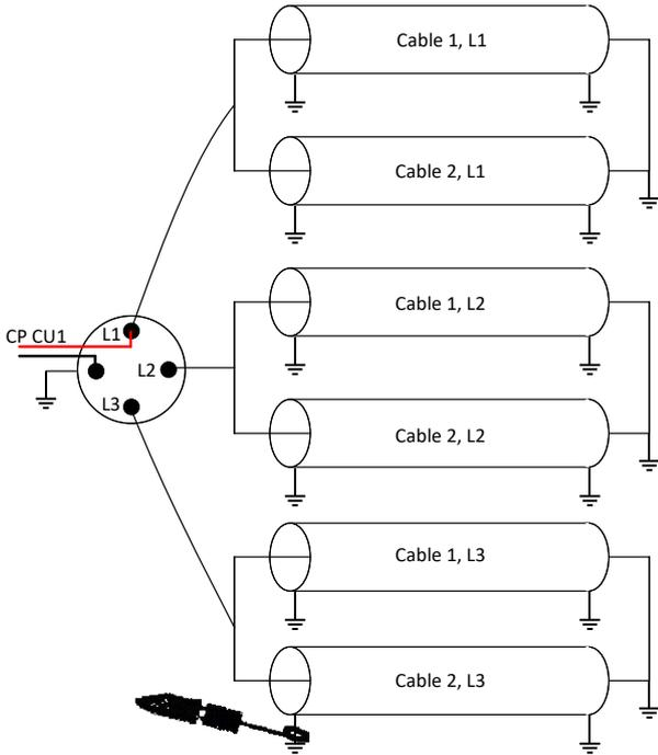
Figure 11 - Feed at L1-E and measurement at shield of cable 2, L3
