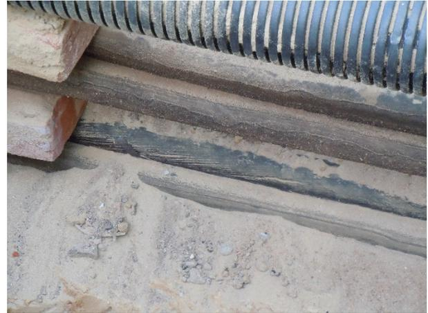
Figure 6 - Shield visible from the outside, the insulation has melted
