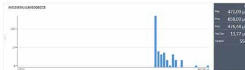
Figure 3: Histogram of propagation delay over (longer) redundant path
