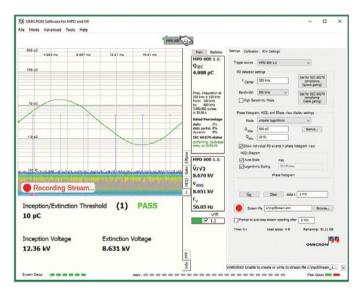
Single-phase PRPD diagram with displayed test voltage and charge value as well as PD inception and PD extinction voltage (MPD 600 Basic Mode)
