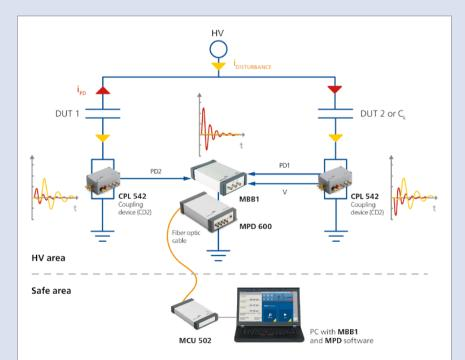
MBB1 measurement bridge For added noise signal reduction in high-voltage laboratories with high interference, the MPD 600 can be used with OMICRON's MBB1 measurement balanced bridge. This accessory can be used to perform differential PD measurements during single-phase AC and DC PD testing. This method provides you with an improved signal-to-noise-ratio and a significant reduction of noise.
