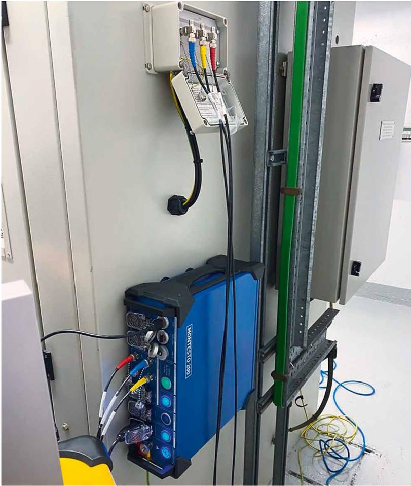
MONTESTO 200 can be easily mounted on the asset for continuous online PD monitoring for longer periods of time.
