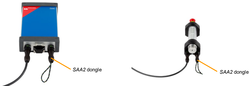
Figure 12: The use of SAA2 dongles
