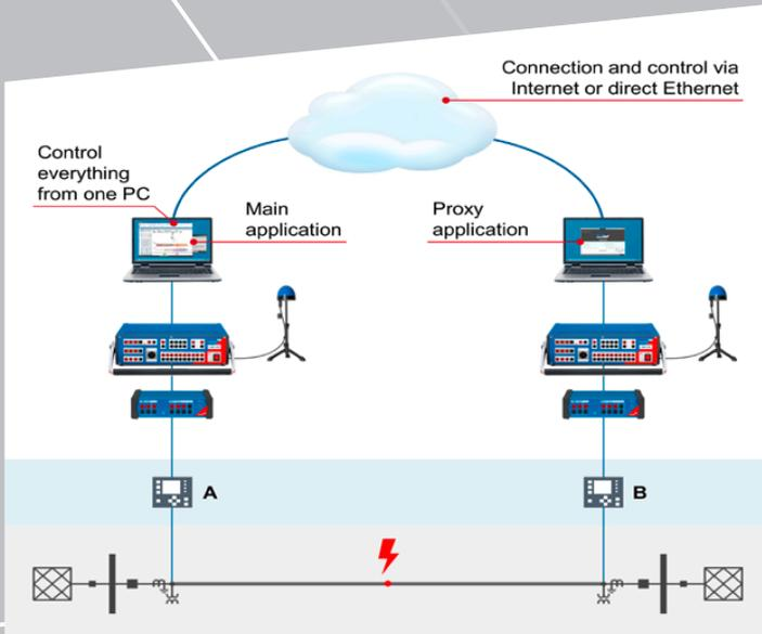
In summation, testing traveling-wave-based relays does not require a new test set, just the TWX1 accessory to expand the scope of your CMC and you are fully prepared, even for the next generation of protection relays.
