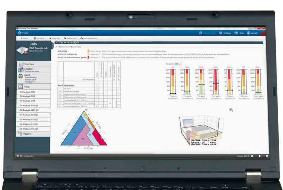
For a comprehensive analysis, PTM offers automatic result assessment and comparison, e.g., of DGA results using interpretation methods such as Duval's traingles.
