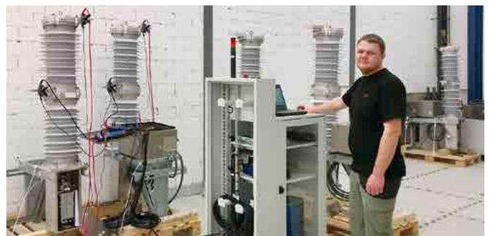
CIBANO 500 test trolley at ABB production line on medium-voltage vacuum CBs.
