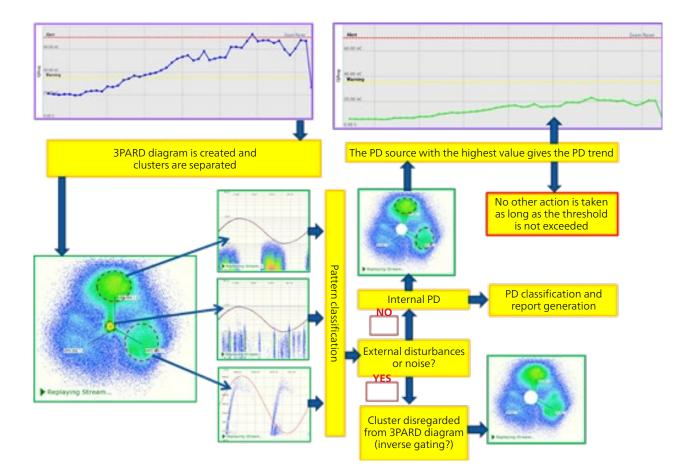
Figure 3: Schematic approach of the entire process between measurement and automated interpretation of the results.
