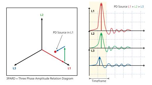
Figure 1: Principle of 3PARD. The simultaneous measurement of the three signals on the right-hand side determines the length of the amplitude vector. The vector sum is the resulting point for this impulse in the 3PARD diagram on the left.
