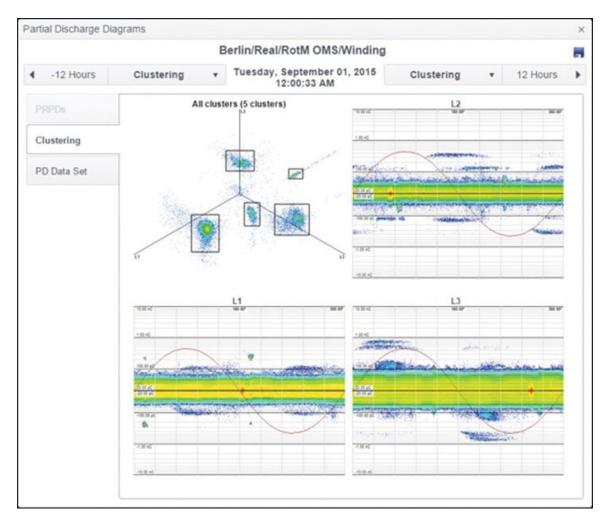
Figure 2: Automated cluster separation. The PRPD diagram and the correlating 3PARD diagram are displayed in this view. The rectangles around the clusters are identified automatically.
