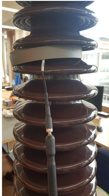
Figure 10: Images Demonstrating How to Set Up a Hot Collar Measurement
