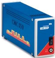
The CMC 850 is OMICRON's protection test set dedicated to IEC 61850. It focuses on the real-time communication methods of GOOSE and Sampled Values to interface with the devices under test. The test set works with the proven Test Universe software and offers even more useful functions embedded directly in the device.
