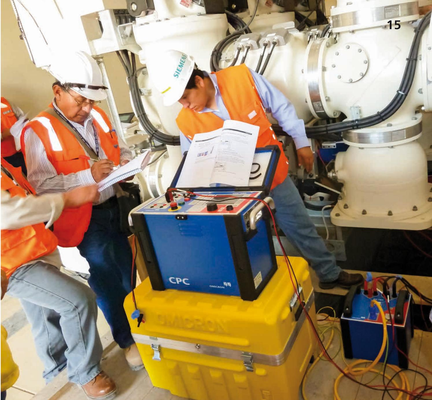
Testing a 72.5 kV type 8DN8-4 GIS in Peru with the CPC 100 + CP RC test system.
