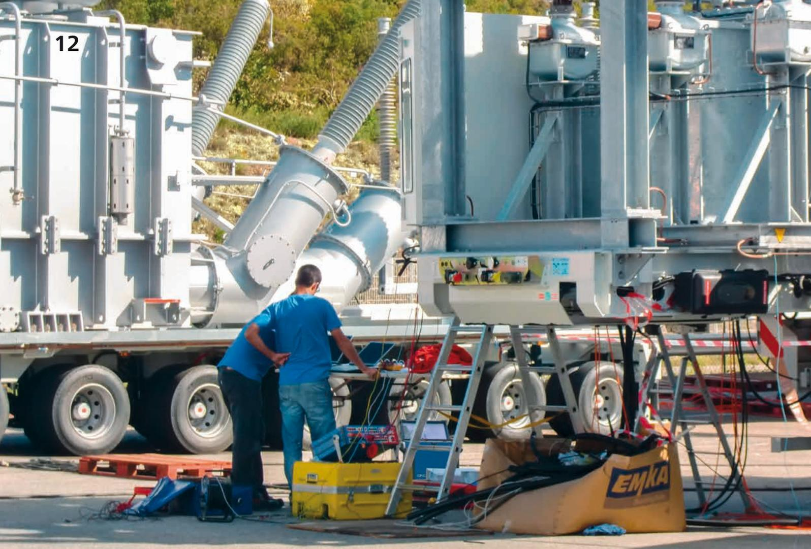
Standardized testing of a 220 kV mobile substation for a project in Algeria with the CPC 100 and the CMC 356.
