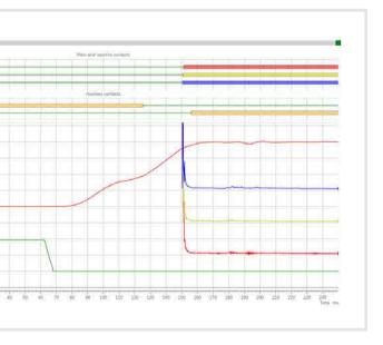
The Primary Test Manager™ software shows the results of the timing measurement using CIBANO 500 and the CSM method.
