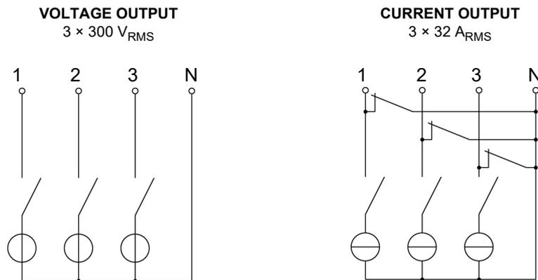
All voltages and current generators can independently be configured with respect to amplitude, phase angle, and frequency.
