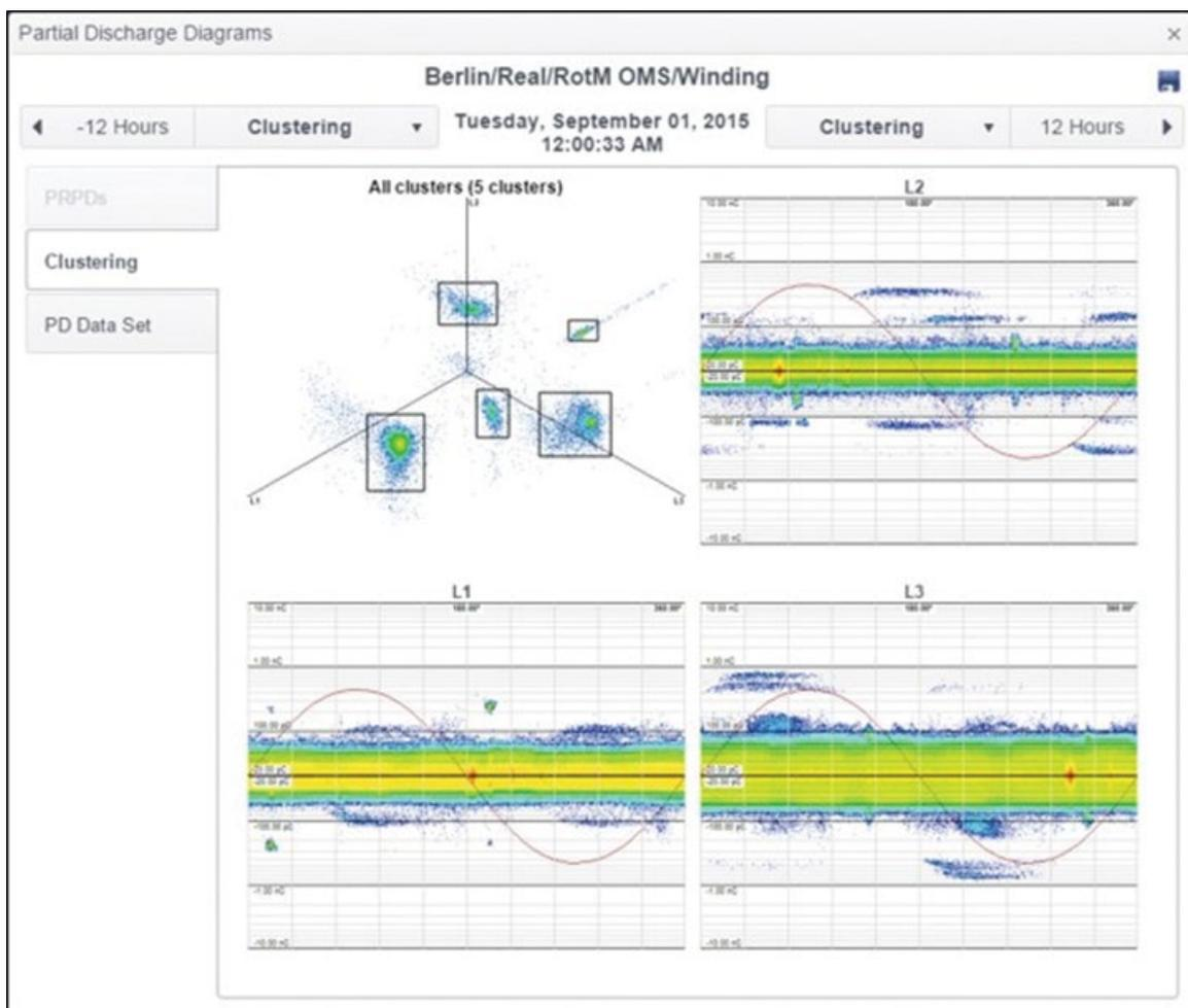
Figure 2: Automated cluster separation. The PRPD diagram and the correlating 3PAR diagram are displayed in this view. The rectangles around the clusters are identified automatically.
