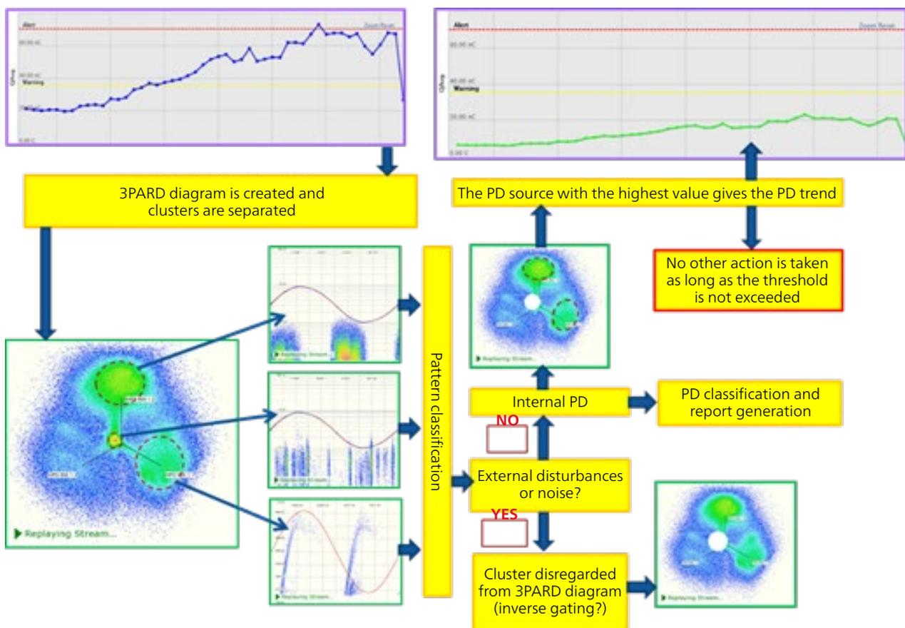
Figure 3: Schematic approach of the entire process between measurement and automated interpretation of the results.
