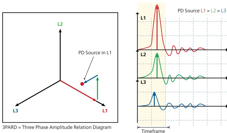
Figure 1: Principle of 3PAR. The simultaneous measurement of the three signals on the right-hand side determines the length of the amplitude vector. The vector sum is the resulting point for this impulse in the 3PAR diagram on the left.
