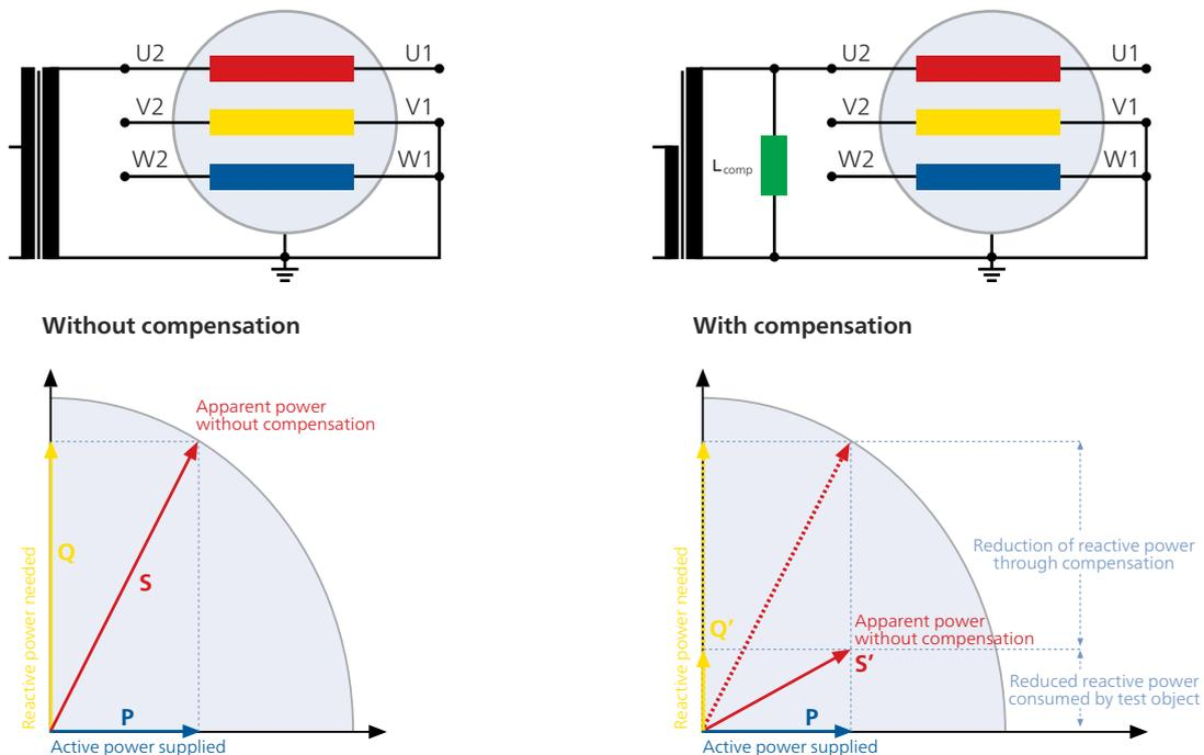
Figure 2: Simplified diagram of compensation with reactor
