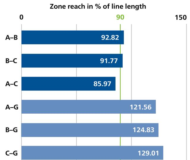
The per mile/km X value of  $Z_1$  is required in order to evaluate the fault locator's accuracy. In this example a fault at 100% of the line length is examined which means, that the fault should correctly be seen at 4.4 mi / 7.1 km.
