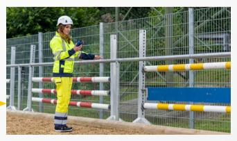
Step- and touch voltage measurement with the handheld meter HGT1
