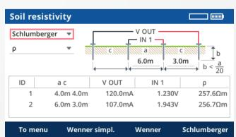
COMPANO 100: Direct calculation of the soil resistivity using the Wenner or Schlumberger method.
