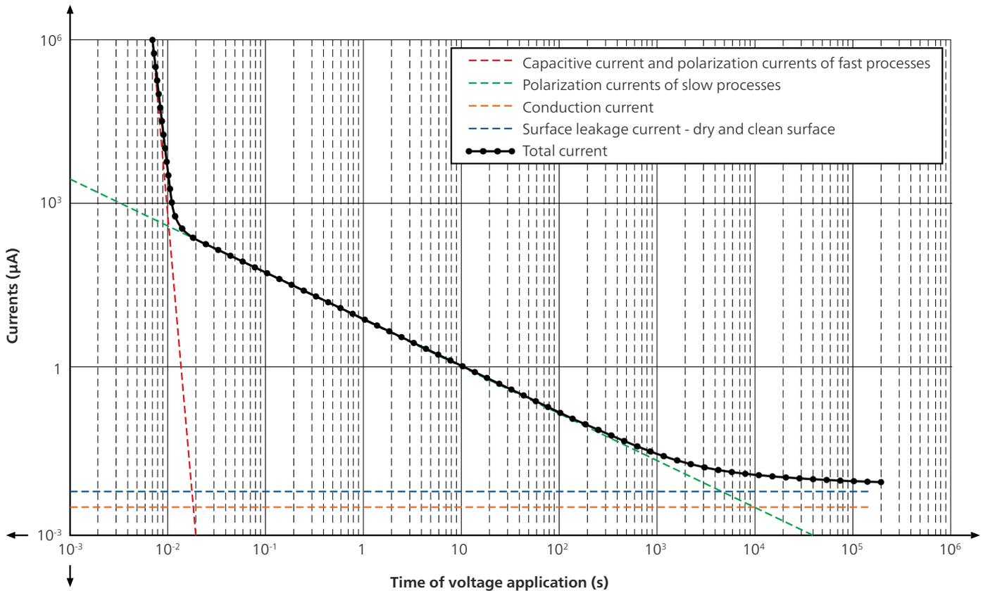
Figure 1: Relative current over time of voltage application. Typical behavior for a synthetic resin based dry and clean winding (the scales are logarithmic); Source: IEC 60034-27-4:2018
