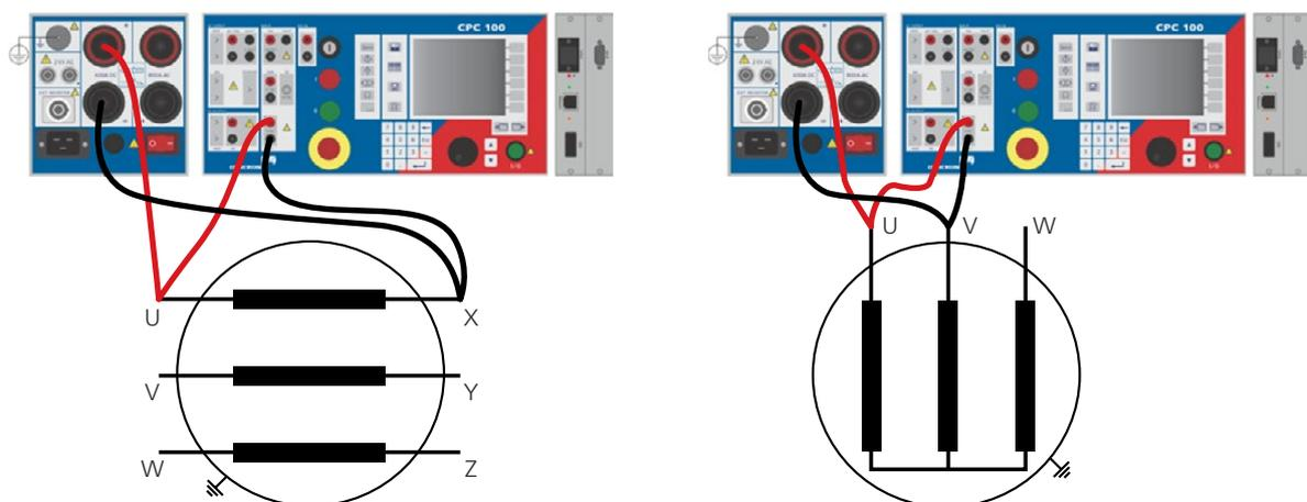
Figure 2: Four wire DC winding resistance measurement on stator winding with open star point (left) and closed star point (right).
