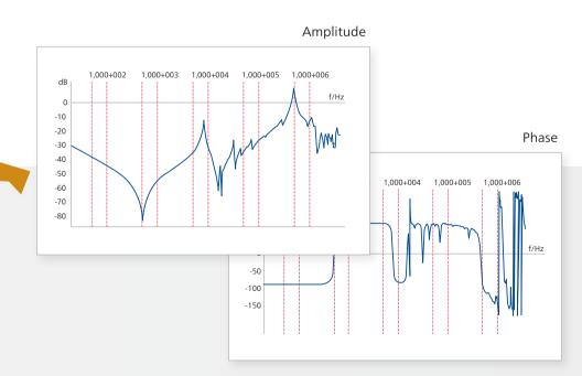
Geometrical changes within and between the elements of the network cause deviations of a transformer's frequency response. FRANEO 800 compares such measurement results with the original fingerprint.
