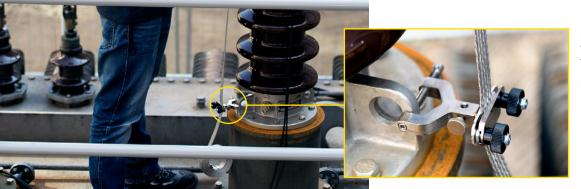
Flange-screw clamps with spikes function as reliable contacts even through layers of paint or dirt.
