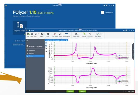
Our PQlyzer software provides optimal support for measuring the transfer characteristics of instrument transformers using configurable sweep settings, wiring diagrams, and reporting for easy use.
