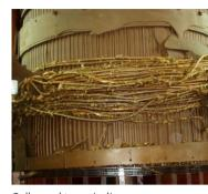
Collapsed tap winding
