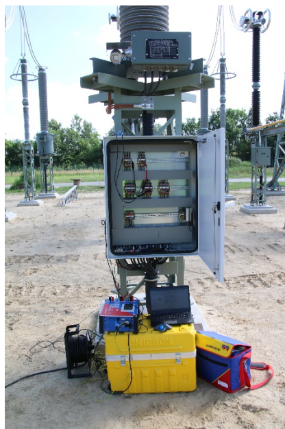
Fig. 5: Measuring configuration of the CT analyzer in the field
