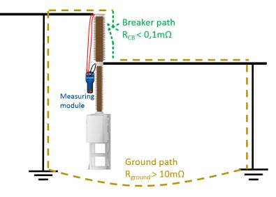
Figure 8: Testing DRM with both sides grounded
