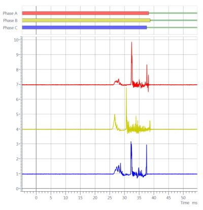
*Figure 7: Current variations (A/s) ever time through each phase during open operation of a 145 kV GIS circuit breaker*
