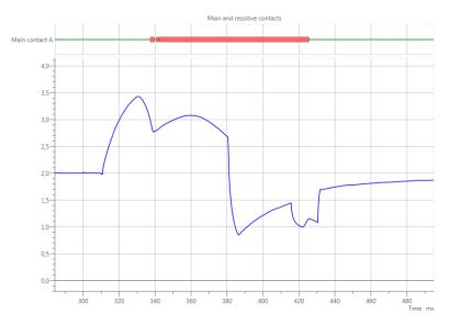
Figure 3: Actuating coil current over time in a CO sequence for a 2kV breaker
