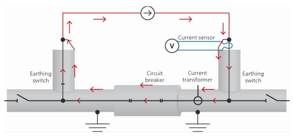
Figure 6: Rogowski coil (current sensor) through earthing switch shunt on a GIS grounded on both sides
