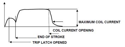
Figure 1: Typical coil current shape
