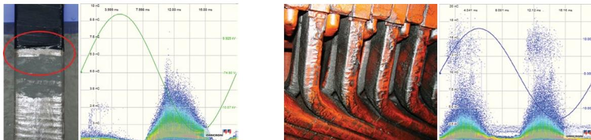
Figure 3: Potential issues in a rotating machine insulation system with correlating PRPD diagram. The left cause represents a disconnected end potential grading from the outer corona protection. The right one represents a polluted endwinding area and the resulting surfaces as well inter-phase discharges.
