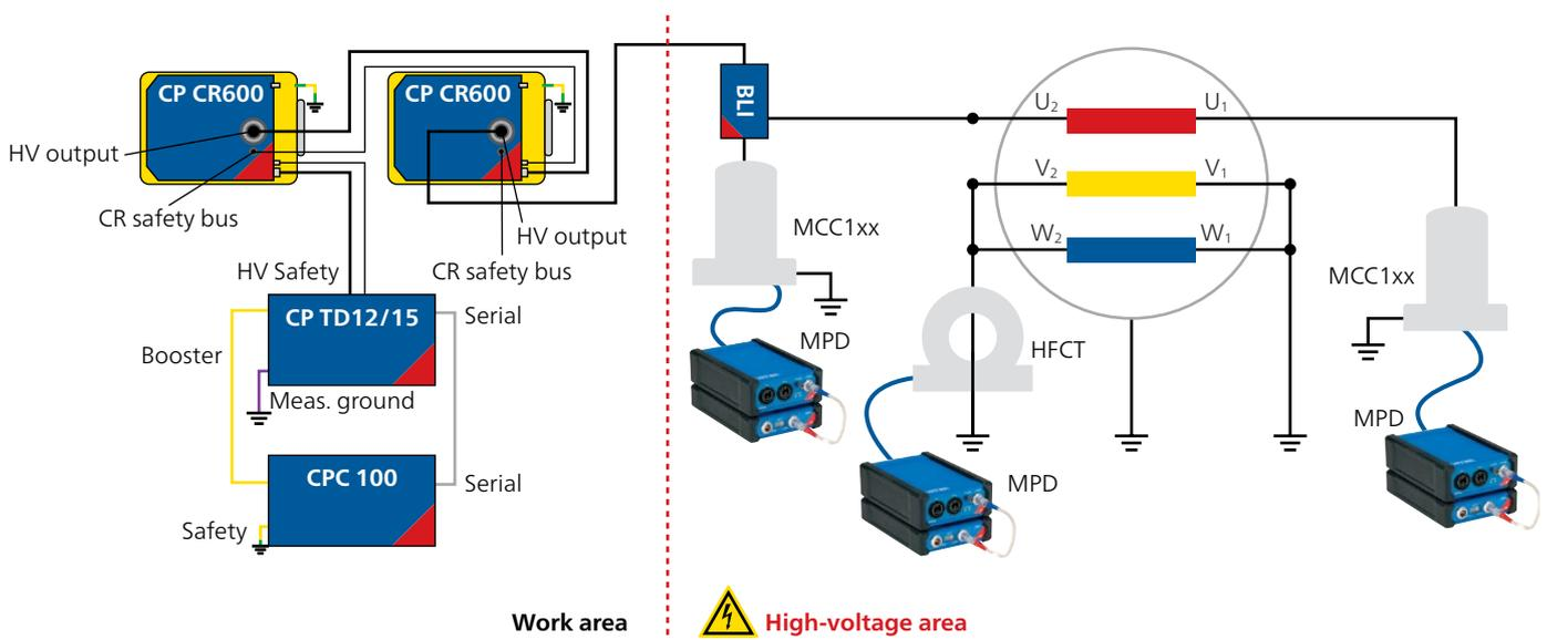
Figure 2: Multi-channel synchronous measurement on a rotating machine
