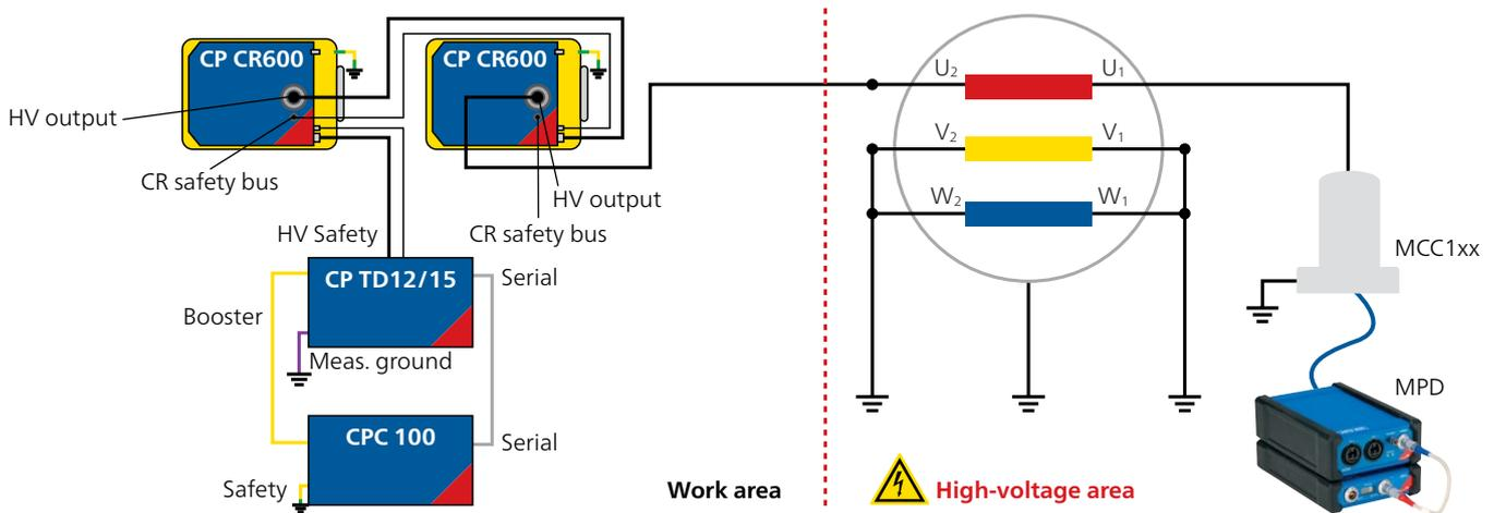
Figure 1: Basic setup for PD measurement on open star rotating machine
