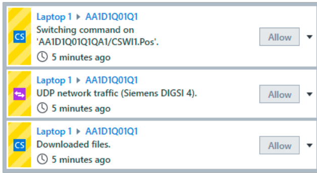
Figure 6: Details for Figure 5: Freshly connected unknown laptop attempting unauthorized control of circuit breaker
