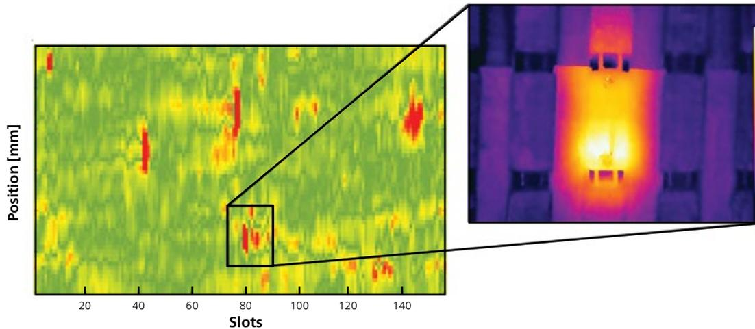
Figure 4. Comparison between a stray flux measurement of an entire stator and a section during a rated flux test on an old, decommissioned stator. The red areas indicate spots with fault currents higher than 100 mA measured during the stray flux measurement.
