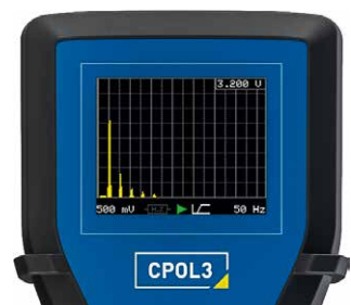
Spectrum mode (FFT) for detecting coupled signals
