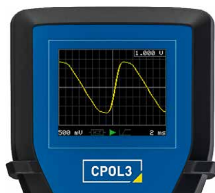
“Oscilloscope” mode for displaying the signal waveform
