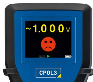
Indication when the test signal polarity is incorrect
