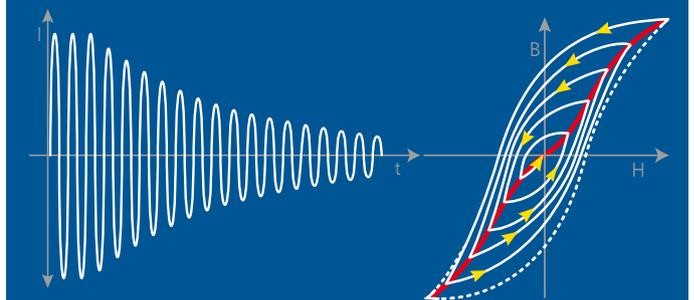
Demagnetization principle of iron cores
