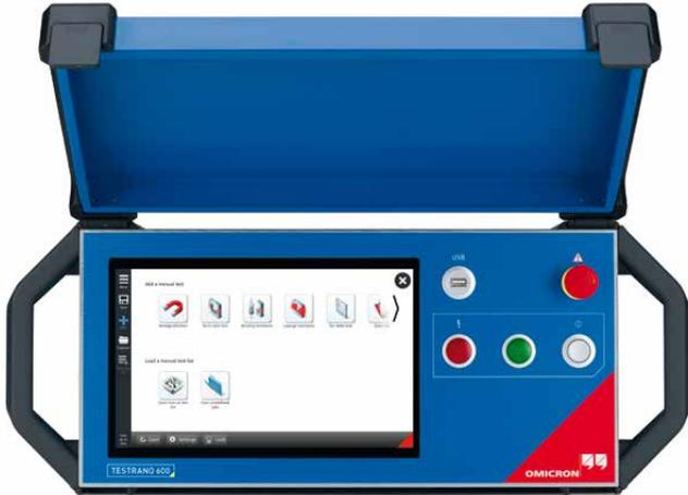
TESTRANO TouchControl on the integrated display offers pre-configured wiring diagrams and convenient features for graphical comparisons and detailed analysis. You can prepare complex tests in advance and import the test files via the USB interface. The high contrast of the high-resolution, multi-touch 10.6" display ensures good visibility even in bright sunlight. This allows fast, flexible and easy testing on site – just touch & test.
