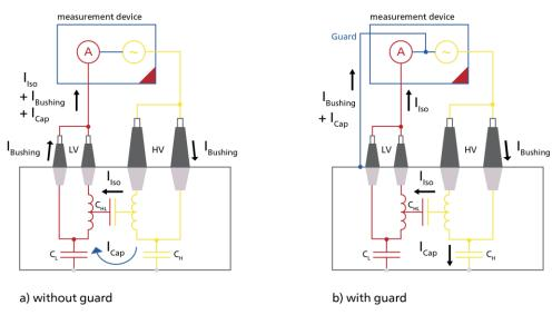
Figure 3: CHL measurement on a 2 winding transformer without and with guard
