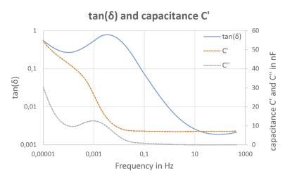
Figure 9: Correlation of the "hump" in tan(δ), the real part C' and the imaginary part C' of the capacitance for a power transformer
