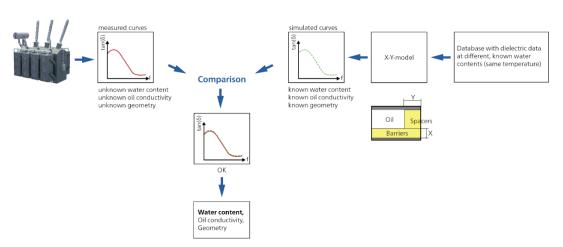
Figure 5: Principle of the water content assessment of power transformers
