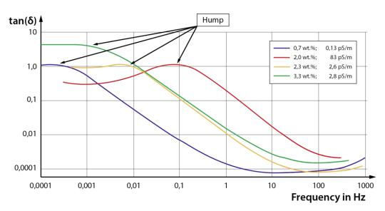
Figure 4: Broadband dielectric response of four different power transformers at 20°C
