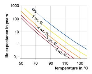
Figure 2 Dependency of life expectance on moisture content and temperature [1]
