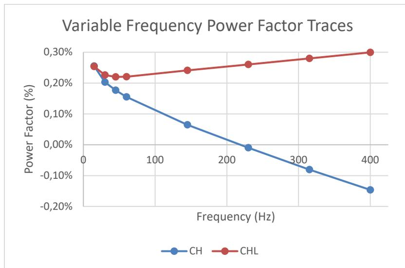
Figure 2 - Variable Frequency Power Factor Results for a Kuhlman 118kV transformer
