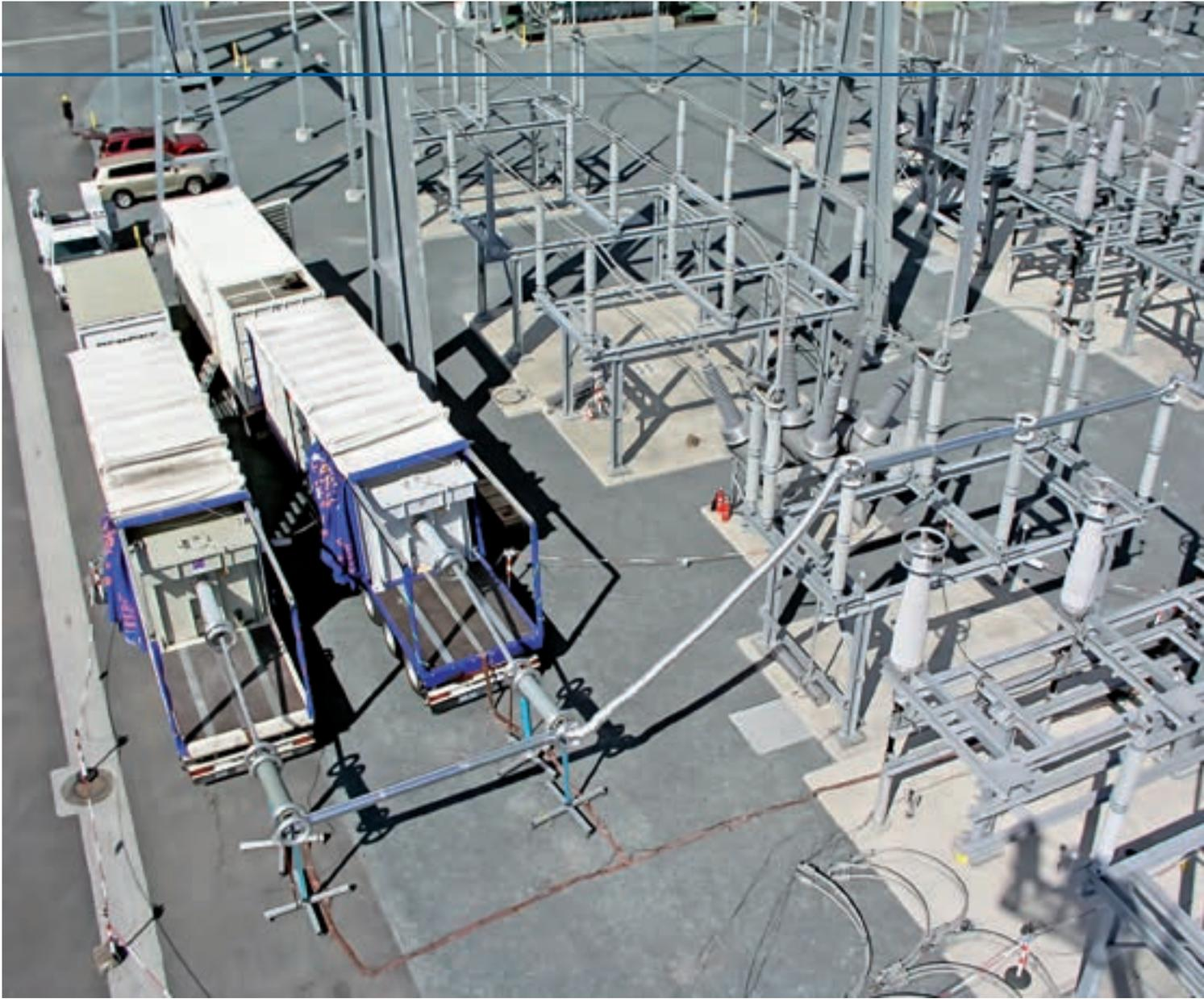
HIGHVOLT testing systems can be connected in parallel with minimal additional effort.
