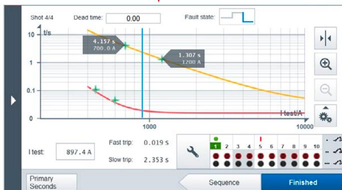
Once the sequence is complete with all test shots, a graphic displays the shots recorded compared to the nominal time.
