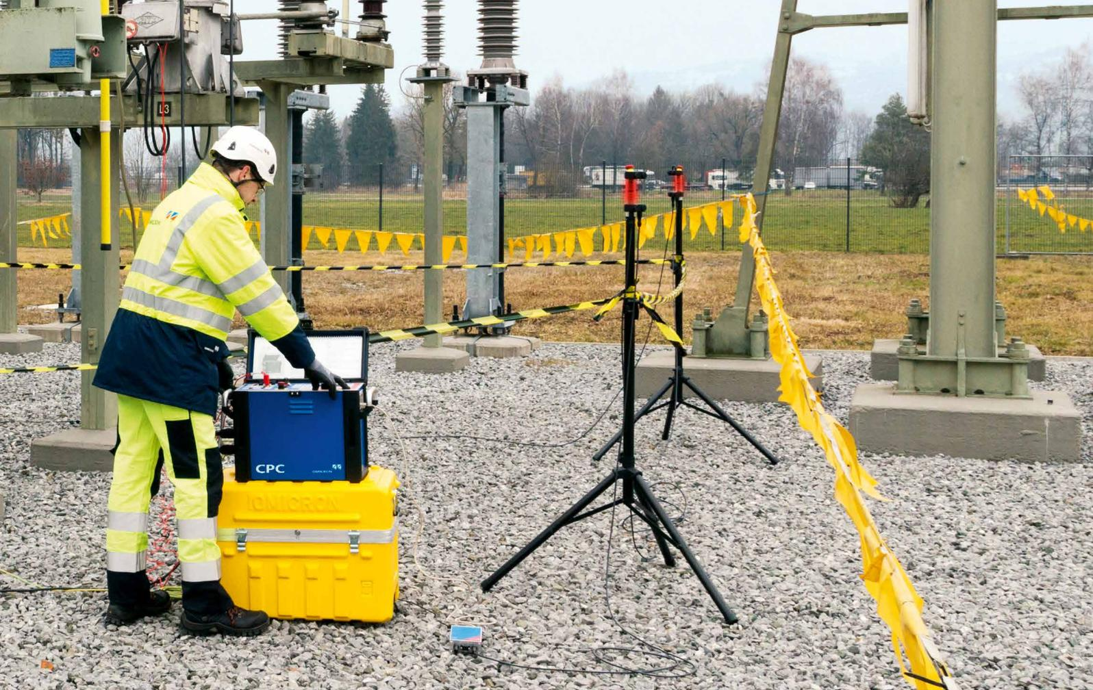
SAA2 in use onsite during transformer testing.
