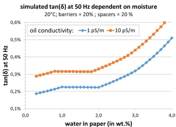
Figure 3. Simulated dependence of the dissipation factor at 50 Hz for a power transformer at two different oil conductivities (simulated  $\tan(\delta)$  at 50 Hz dependent on moisture; 20°C; barriers = 20 % , spacers 20 %; oil conductivity 1 pS/m, 10 pS/m;  $\tan(\delta)$  at 50 Hz; water in paper (in wt.%)
