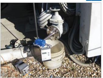
Drain valve sensor for insertion temporary into the transformer for UHF PD measurement
