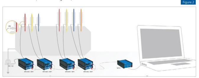
Conventional PD measurement on an HV bushing without measurement taps
