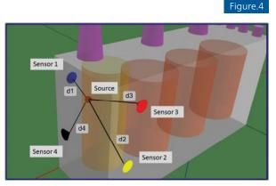
Principle of acoustic PD localization with external sensors
