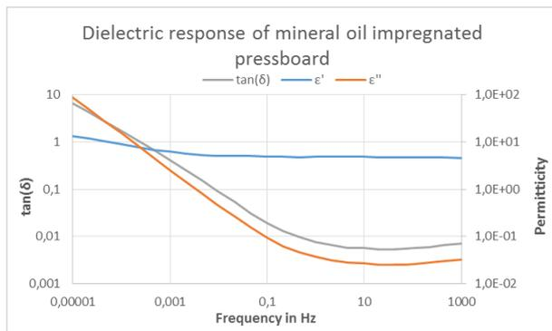
Figure 4: Dielectric response of mineral oil impregnated pressboard.
