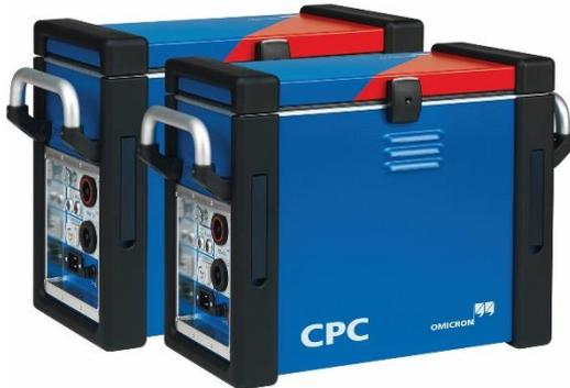
CPCSync enables users to easily synchronize up to three CPC 100 devices to create an HV source with up to 15 kVA.
