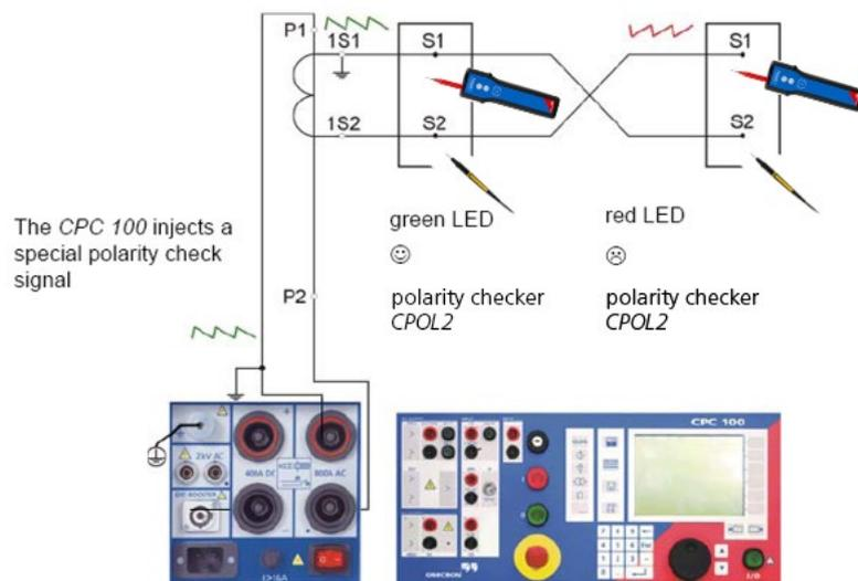
**Fig. 6:** Wiring testing with the CPOL2
