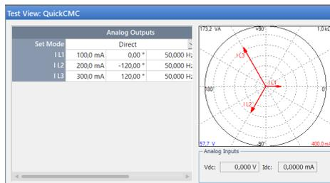
**Fig. 1:** Asymmetric injection with the QuickCMC
