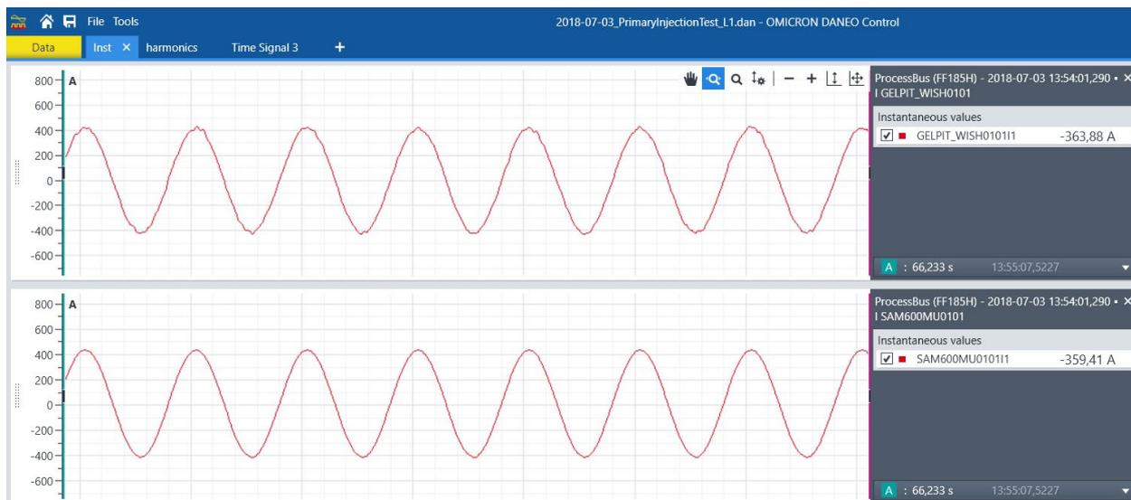
**Fig. 8:** Signal plot comparison using OMICRON's DANEO 400
