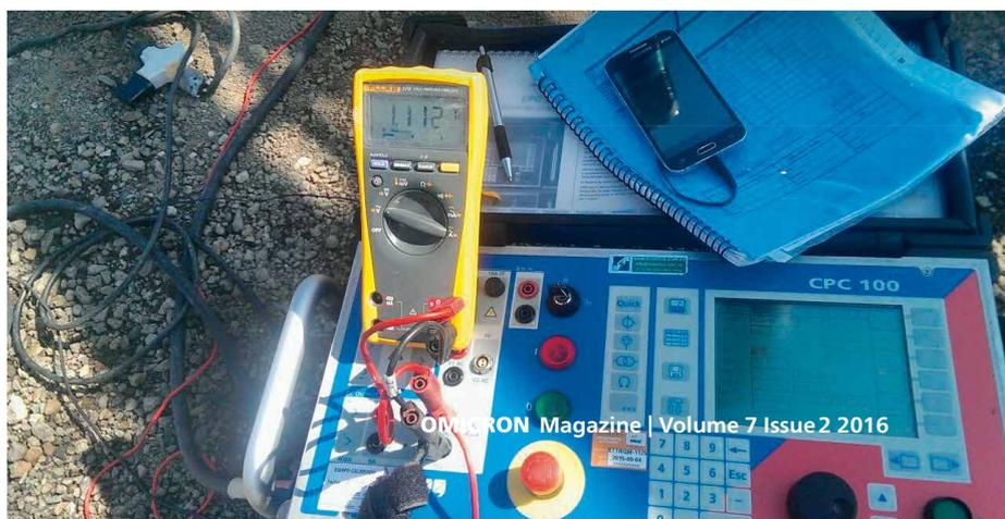
300A DC that was required, a DC voltmeter, a DC clamp ammeter and markers for identifying the test points (Figure 2). The resistances per meter were determined for several test points in the substation as shown in figure 3. The measurement showed no significant deviations between the relative resistances within the substation. All of the values were between 0.4 mΩ/m and 1.2 mΩ/m.
