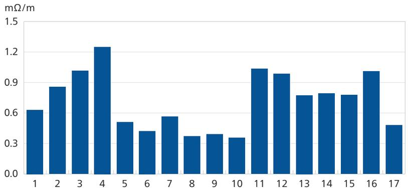
▲ Figure 3: The diagram shows the resistances of the different test points in relation to the distance between the reference point and test point.
