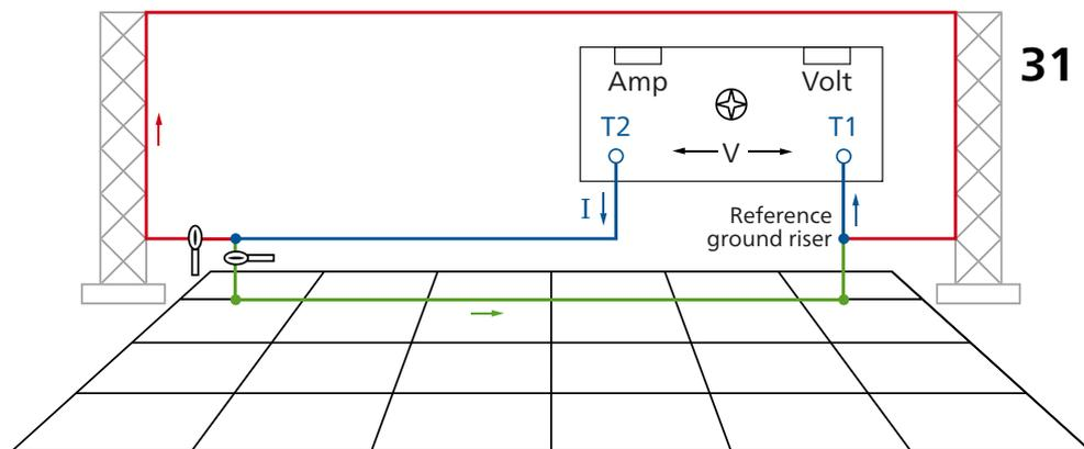
Resistivity, Ground Impedance, and Earth Surface Potentials of a Grounding System" (IEEE 81 standard) different methods for measuring the continuity are mentioned. A 230 kV substation was examined using the 'high-current test method'.
