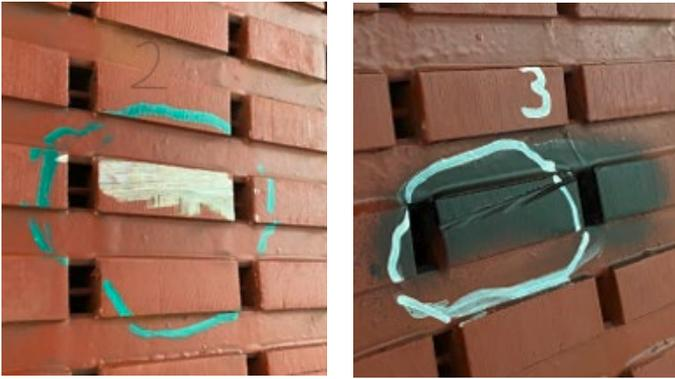
Example of the fault implementation and black painting to avoid reflection during thermographic measurement.
