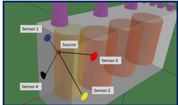
Figure 8: Principle of acoustic localization [18]
