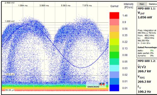
Figure 15: Pattern of this internal PD measured synchronously with UHF technology [22]
