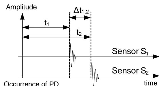
Figure 7: Absolute and relative times in a two-sensor-setup
