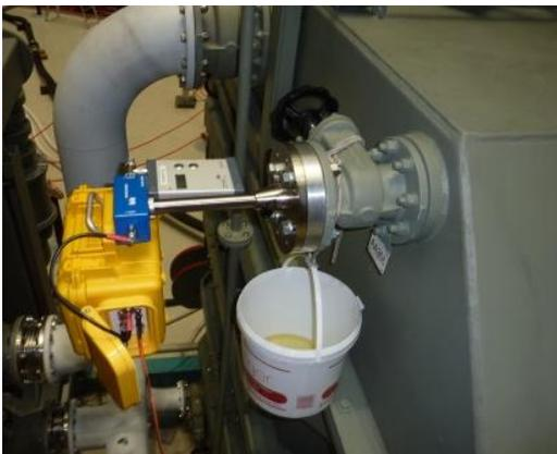
**Figure 11:** UHF sensor connected to the tested transformer in the factory test laboratory
