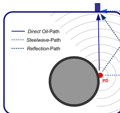
Figure 5: Possible propagation paths in the test object [18]
