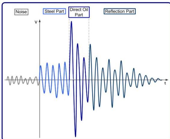
Figure 6: Acoustic PD signal components reflecting the propagation paths
