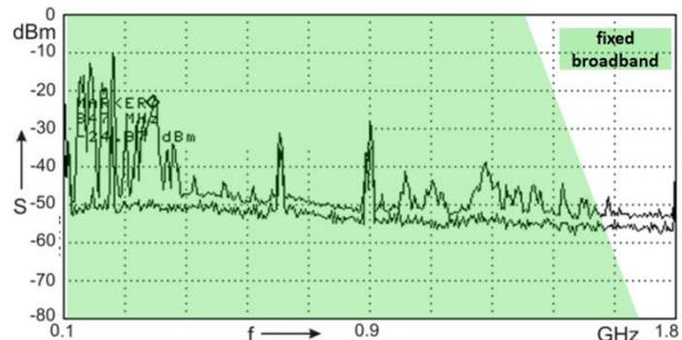
Figure 3: Bandwidth of fixed broadband UHF method (schematic example) [9]
