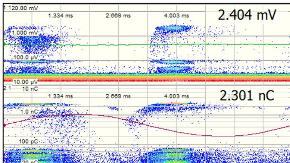
Figure 16: Simultaneously measured PD pattern of the UHF system (top) and conventional PD detector at the bushing tap (bottom)
