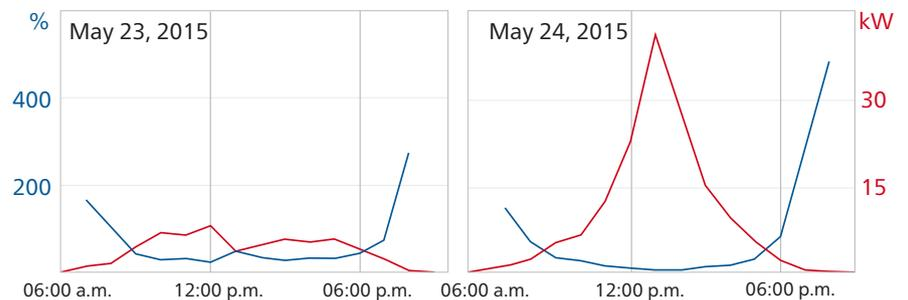
Figure 2: The THD<sub>i</sub> reacted inversely proportional to the output.
