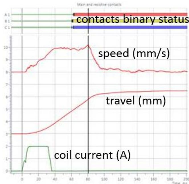
Figure 4: Damping analysis over time
