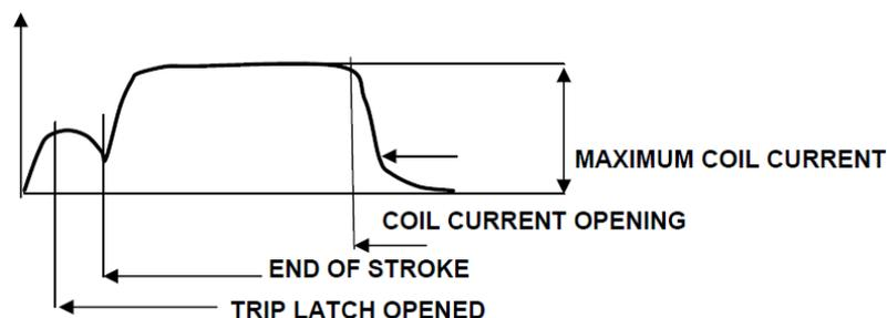
Figure 1: Typical coil current shape
