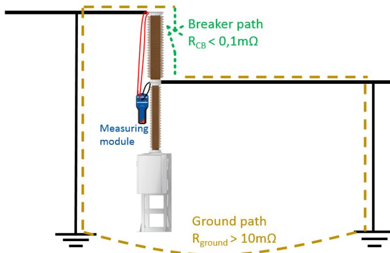
Figure 8: Testing DRM with both sides grounded
