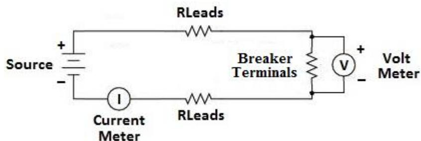
Figure 7 - Kelvin Connection Used for Contact Resistance Measurement
