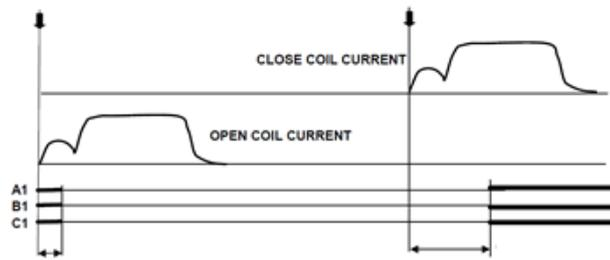
Figure 2 - Command Coil Currents and Main Contact State
