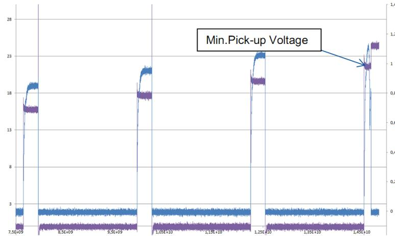
Figure 9 - Minimum Pick: Voltage and Current Responses
