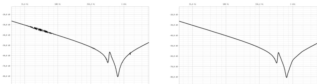
Figure 12. Comparison of the SFRA trace before (left) and after noise removal (right)
