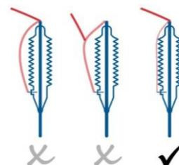
Figure 8: Recommended setup according to IEC 60076-18
