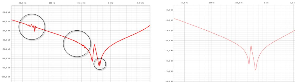
Figure 13: End-to-end open-circuit on HV winding performed with SFRA Instrument 1 (left) and SFRA Instrument 2 (right)
