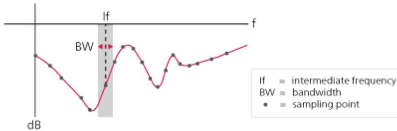
Figure 10: Illustration of the adaptive bandwidth concept
