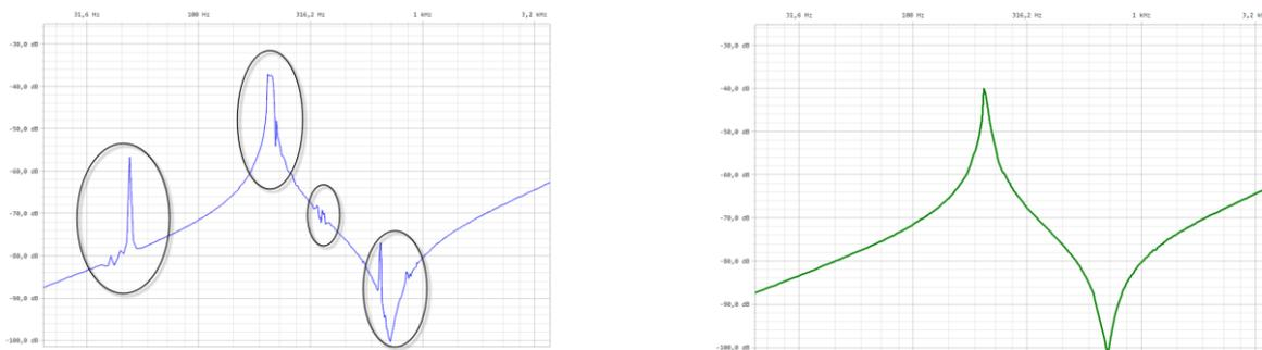
Figure 14: Capacitive interwinding on HV winding performed with SFRA Instrument 1 (left) and SFRA Instrument 2 (right)
