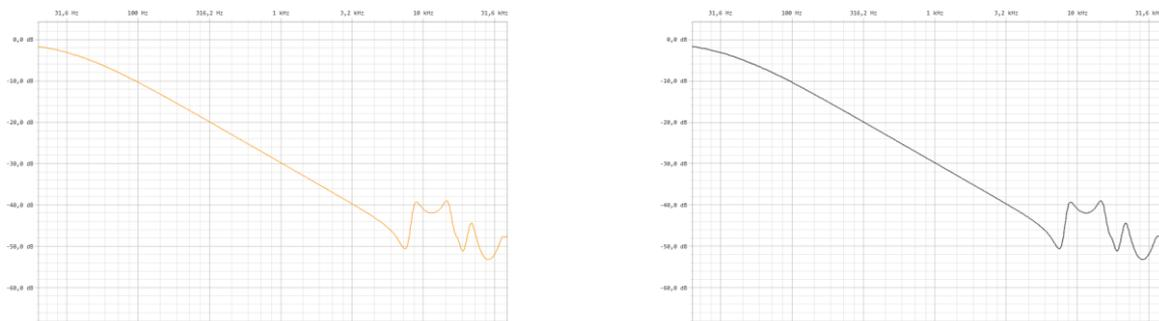
Figure 15: End-to-end short-circuit on HV winding performed with SFRA Instrument 1 (left) and SFRA Instrument 2 (right)
